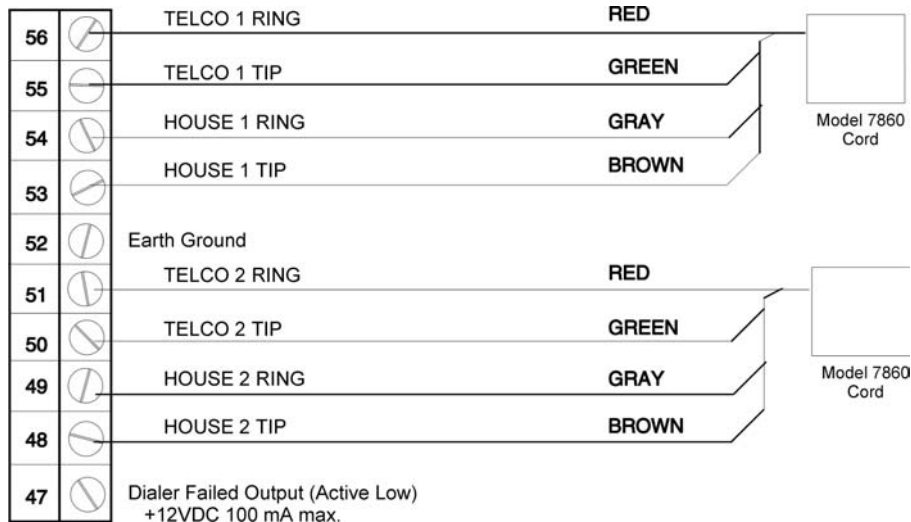
Figure 3-6 Telephone Line Connection
